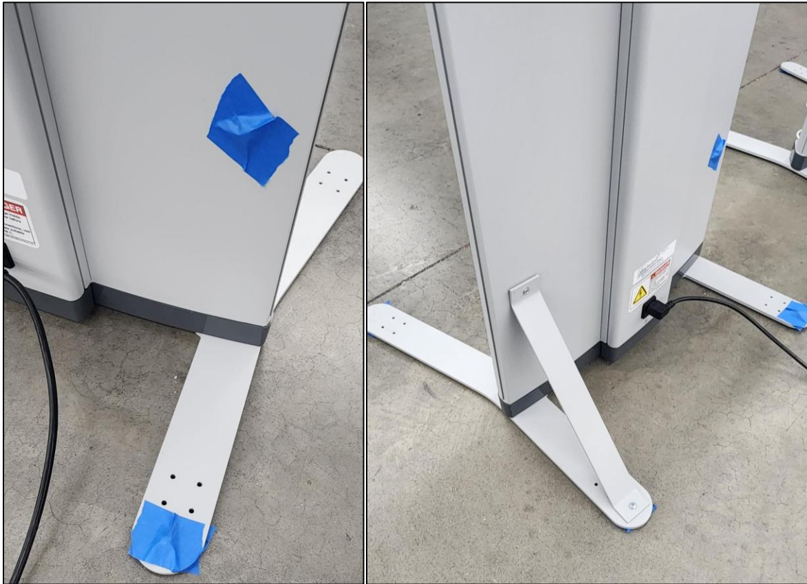
Figure 4 Left – Stabilizer screws covered by tape. Right – Stabilizer mounted.
