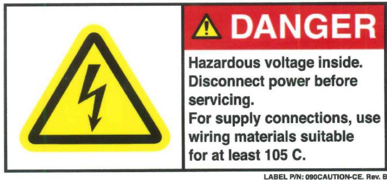
Figure 7 Hazardous Voltage Label
