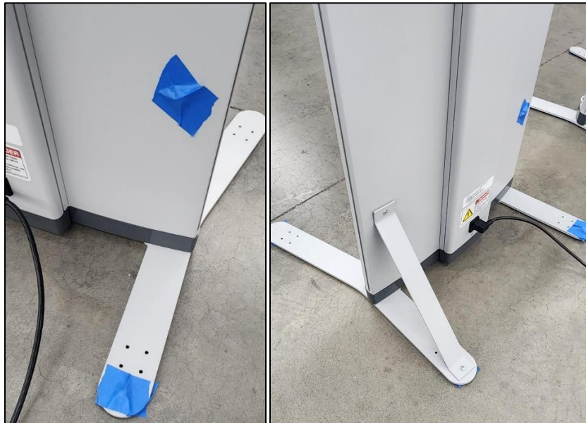
Figure 2 Left – Stabilizer screws covered by tape. Right – Stabilizer mounted.
